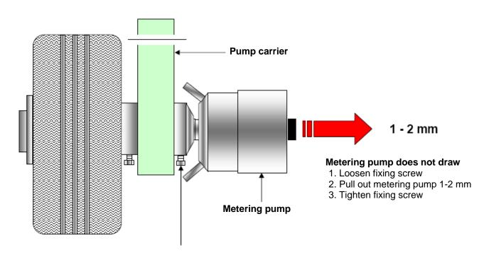
Clamping bush fixing screw
