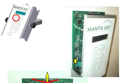
Although voltage is applied to the control box, it can not be switched on. There could be two reasons. One reason is a faulty keyboard. The other reason is the cable between the keyboard and motherboard. By opening the control, this compound have been disconnected and needs to be reconnected.
