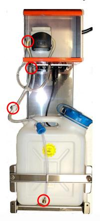
If the device has already been in operation, particles can block the hose directly to the hose locking device. In this case, open the quick-coupling and allow the pump to run backwards to remove the blockade. Any restriction (pictured in red) can lead to a blockade in worst case. These points should be checked first if the pump suddenly got no output, but the engine is still running.
