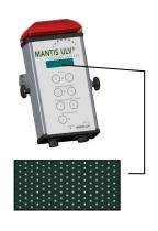
After switching-on the control box the display gives no information
