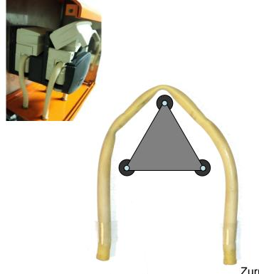
The pump hose is subjected to an aging process. High speeds, aggressive fluids and UV radiation decreases the resilience of the tube and the performance of the pump is reduced.
