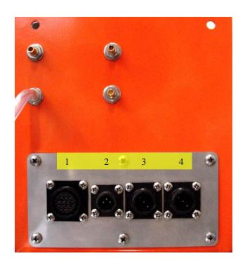
If you have a MAFEX Potato /1 and neither of the two atomiser ports at the pump box is closed with a lid, then switch once the connections between positions three and four.
