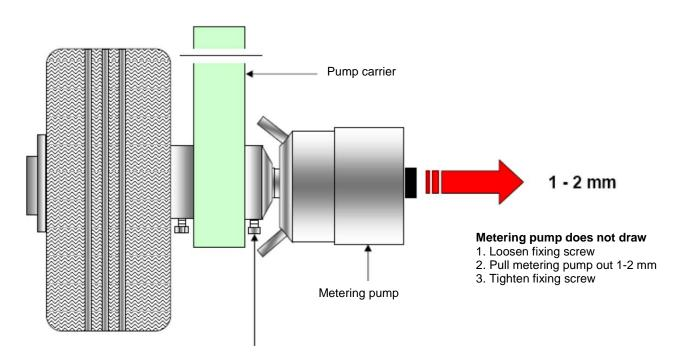
Clamping bush fixing screw
