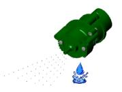
The atomiser sprays not the full width and dripps
